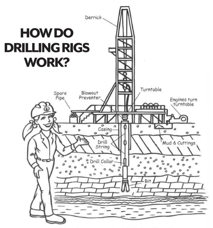
Drilling Rigs are used to drill deep into the earth's natural formations to reach oil and gas.
